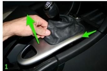
•First, we need to get access to the bushings. They are at the base of the shifter housing. (The black plastic part.) Lift up and slide back the shifter cover to get it out of the way. Img 1.
