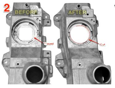
• Modifying the base. (Fig. 2) After cutting the template and marking the base you will need to cut the base out. Die grinder works ok. Make sure to remove all the burrs and shavings when you are done.
