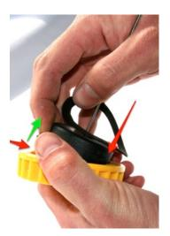
3. Once the seal ring is out, press down on the black plastic below one of the keeper tabs (Large red arrow to left) and rock the assembly out by pulling up on the other
