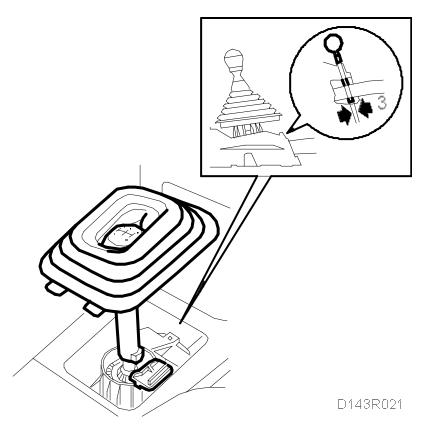
If the locking pin cannot be inserted, the gear position needs adjusting as described in step 4 to 10 below. Remove the locking pin if no adjustment is required.
