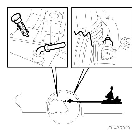
2. Remove the plastic plug on the gearbox and insert <u>87 92 335 Locking pin</u> to secure 4th gear in the gearbox.
