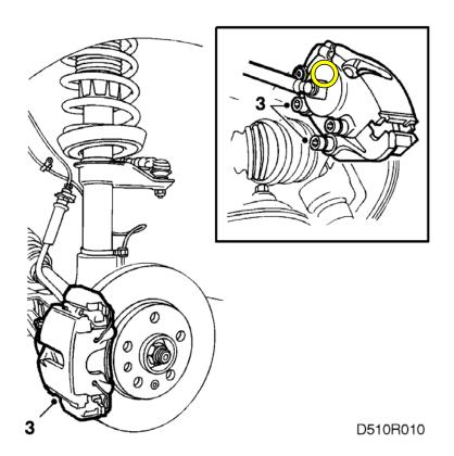
Tightening torque 118 Nm (87 lbf ft)
