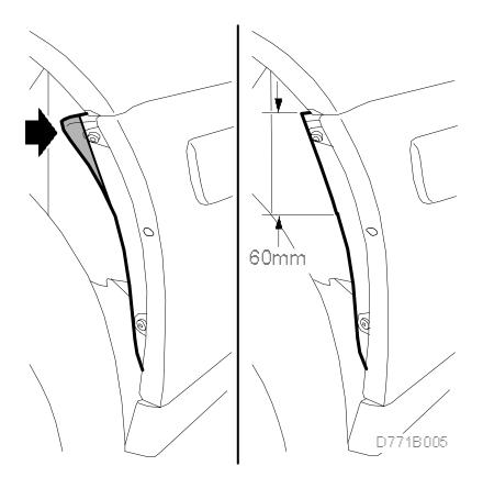
2. Remove the plastic nuts from the two lower bolts in the wheel housing behind the front wheel.
