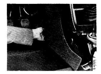
8 Remove the securing screws and slide back the rear air duct.
