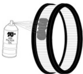
After cleaning air filter always re-oil before using. Spray K&N air filter oil down into each pleat with one pass per pleat. Wait 20 minutes and re-oil any white spots still showing.
