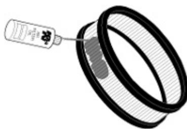
After cleaning air filter always re-oil before using. Squeeze K&N air filter oil down into the bottom and along each pleat in only one pass per pleat. Let oil wick into cotton for 20 minutes. Re-oil any white spots still showing.
