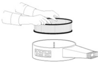
Re-install your K&N air filter element with proper care. Make sure the element seats properly in the filter case. Install the cover making sure it's in the right position. Tighten all the nuts, bolts, screws or clips to factory specifications.
