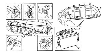
Next you need to remove the 4 10mm hex nuts that hold down the rubber boot of the weather proofing (Item 7) the rear two are a bit hidden. Be careful to not chip the edge of the windshield with the ratchet. Once loosened the boot can be slid up the wire harness to give necessary room. (Image to the right) Remove the electrical connector by lifting the lock lever up and to the drivers side.
