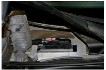
When replacing the ecu be sure to bolt it in the right way round to that the electrical connector will fit.
