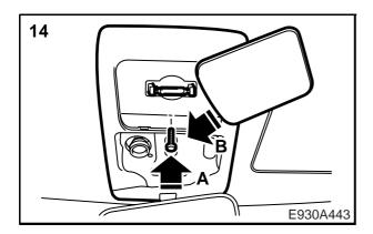
14 Press the cover in, fit the retaining screw (B) and the glass cover (A).
