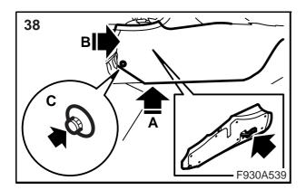
38 Fit the floor console's right-hand side piece.
