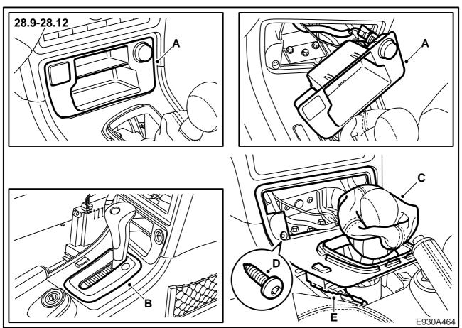
28.9 Plug in the connector (E) and fit the cover's screws (D).
