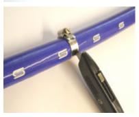
Holding the hose securely, away from the point of intended cutting, make an incision with the knife at a position at the side of the hose clamp band. Slowly cut along the edge of the hose clamp band to obtain a straight cut.
