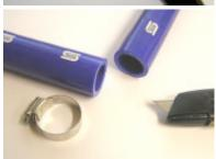
Once the cut has traversed the circumference, remove the hose clamp.
