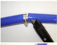
Due to an uneven edge near the adjuster of the clamp, it is advisable to stop before reaching this position, slacken and rotate the clamp, re-tighten and continue your cut around the circumference.
