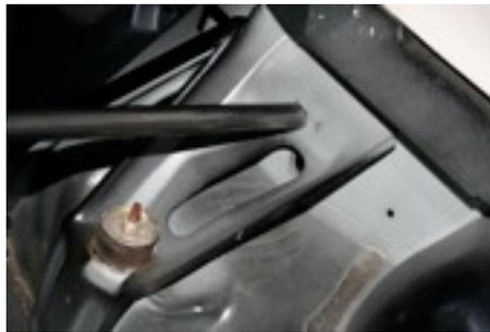
5. Once the brace is somewhat in place with the bottom hanging free you can reach under the speakers and start the 12mm screws in the side making sure the reinforcement washers are under the head. You may find it easier to reach through from the front side too. Just run them down close for now we will final tighten them later.
