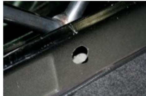
Switch back to the 3/8 and drill completely through both layers of the body.
