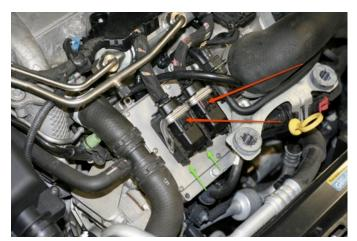
2.The electrical connectors (Red Arrows Left) are a little tricky since they can stick a bit. Do not use a screwdriver to pry on them or you risk breakage. Push down on the safety tab (Red arrow) releasing the silver lock lever. At the same tie you are lifting the lever you may need to help the clip slide by pushing on the lock itself. (Green arrows) The connector will slide open and can be lifted out of the way.
