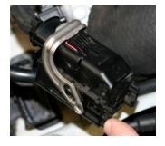
3. Show to the far left is locked closed. To the right is the connector in the open position
