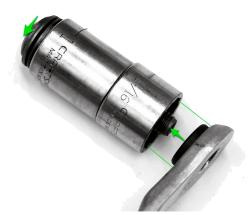
• Preferred Method, the easiest method is using the stock bolt, a couple washers and assorted sockets to pull the insert out. of the original arm. You need to make sure you have a large enough socket to clear the threaded insert but still seat solidly on the arm. We use a1/2" Drive 1-1/16" 12 point socket. Using the mechanical advantage of the screw makes this the easiest method. We use this in the shop for all the upgraded arms that go out.
