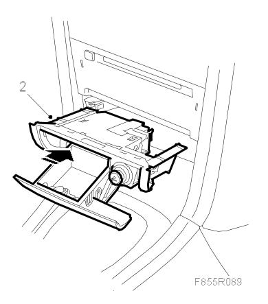
3. Check that the locking clips engage on both sides.
